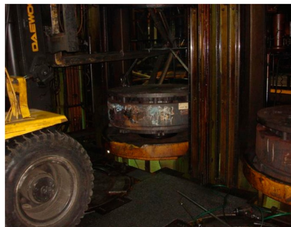
Figure 1 A worker is transferring and placing a mold by using a forklift.
