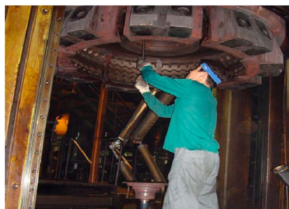
Figure 2 A worker is assembling a mold without any respiratory protective equipment.
